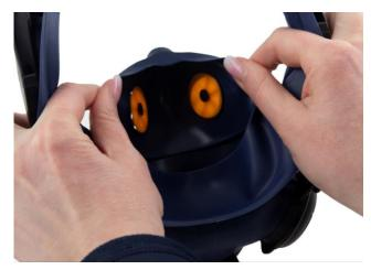
**13.2** Two membranes are fitted, i.e. one on each inside of the inner mask. The dowels for these membranes are removable and should be changed whenever the membrane is changed. Prise off the membrane and dowels.
