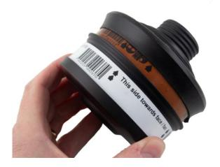
**3.1** During work in atmospheres containing both particulates and gases/vapors (such as spray painting) the particulate filter and chemical cartridge should be combined. Press the filter/cartridge together so that the arrows on the particulate filter point towards the chemical cartridge.
