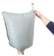
**2.1** Place the facepiece in the bag and grip the opening of the bag so that it seals around the breathing hose. Grip the flow meter with the other hand and hold it so that it points vertically up from the bag.
