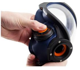
**14.4** Press the valve covers into place. A clicking sound indicates that the cover has snapped into place. Carry out leakage testing.
