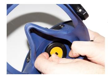
**13.1** One membrane is in the centre of the inner mask on a fixed dowel. Prise off the membrane and fit a new membrane.
