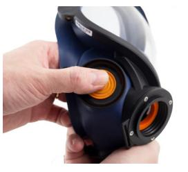
14.3 Press the new membranes onto the dowels.Carefully check that the membranes are in contact with the valve seats all round.
