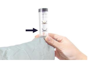
**2.2** Read the position of the ball in the tube. It should float level with or just above the marking on the tube.
