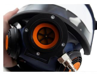
**1.2** The membranes are consumables and must be replaced if there are any signs of damage or ageing. Check the condition of the head harness. The head harness is a consumable item and should be replaced if there are any signs of wear or reduced elasticity.
