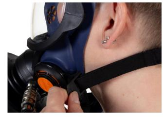
**10.2** Slacken the four elastic straps in pairs by moving the strap holders forward. The two inelastic straps need not be released
