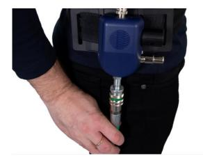
**9.2** Disconnect the compressed air hose from the control valve.
