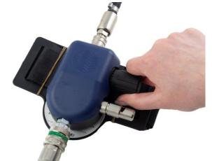
**1.6** Turn the control valve knob anti-clockwise as far as it will go, in order to throttle the air flow rate to a minimum.
