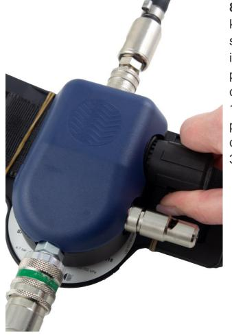
**8.1** Use the control valve knob to set the air flow rate to suit your current work intensity. In the fully closed position (turn the knob anti-clockwise), the flow is about 150 l/min. In the fully open position (turn the knob clockwise), the flow is about 320 l/min.
