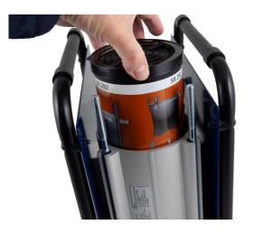
**2.4** Remove the used filter element.
