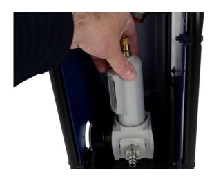
**3.2** Remove the drain bowl. Press it downward and twist anti-clockwise (bayonet mounting). Wash the bowl in hot water (not solvent) at a maximum of 60 °C.
