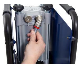
**2.8** Connect the hose between the control valve and filter lid by pushing the hose into the connector.
