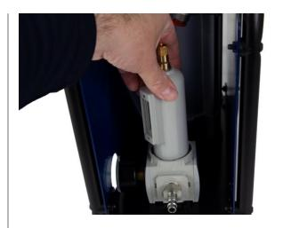
**4.2** Remove the drain bowl. Press it downward and twist anti-clockwise (bayonet mounting). Wash the bowl in hot water (not solvent) at a maximum of 60 °C.
