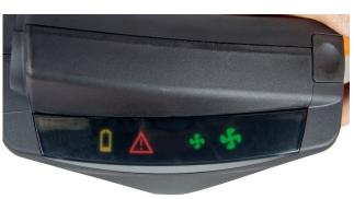
**6.2** After the button has been pressed, a programmed test will be run on the fan and the display will then light up, the audible signal will sound.
