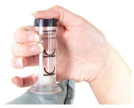
**10.1** Cause a flow stoppage by still holding tightly the joint between the hose and the flow meter bag and then blocking off the flow meter outlet.
