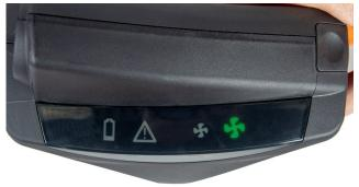
**6.4** If the button is pressed again, boosted operating status will be activated, with a flow at least 225 l/min. This is indicated by the larger green fan symbol lighting up. To revert to normal operation, press the control button once again.
