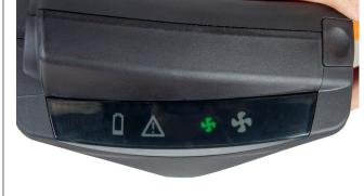
**6.3** After the internal test, all symbols will be extinguished except the small green fan symbol. This indicates normal operating status with a flow of at least 175 I / min.
